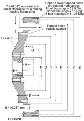
The appropriate standards list tolerances for machined surfaces, threads bore eccentricity and face deviation. Should any of this detail be required please consult our sales staff for a copy of the complete SAE standard. Flywheel shown with pilot bearing installed for reference only. Pilot bearing is required only when using over centre clutches or torque converters. If fitting a flywheel drive plate for hydraulic pump drives, the bearing should
